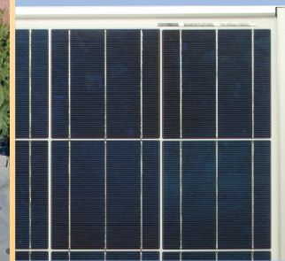
New high efficiency cells each have 3 tabs.
